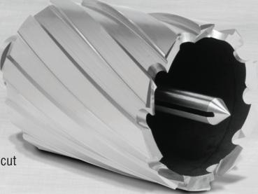
Pilots go through the center of the cutter. They retract up into the mag drill arbor as the hole is made. Pilots last a very long time and can be used with multiple sizes of cutters.
