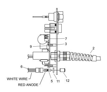
NOTE: WHEN INSERTING L.E.D. DETAIL#5 INTO HARNESS DETAIL#2 MAKE SURE FLAT ON BULB LINES UP WITH WHITE WIRE ON HARNESS.
