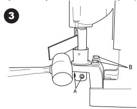
Another method is to use a Dead Blow Hammer and a Flat Metal Bar (refer to dia. 3). With the Magnet "ON" and attached to a metal plate. Insert the Flat Metal Bar into the slot of the Arbor Body. With a Dead Blow Hammer, strike the flat bar quick and firm to shock the Arbor Body loose. Un-thread the Arbor Body completely and remove the bolts from the Magnet (B).
