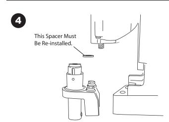
When the Arbor Body Assembly is removed be aware of the Spacer between the Arbor Body Assembly and the Motor Assembly. Refer to the next page to install the 3-Jaw Chuck Assembly.
