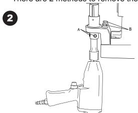
One method is to use an 1/2 drive Impact Gun with a short extension (refer to dia. 2). The extension can be installed into the bottom of the Arbor Body Assembly as a cutter would. Tighten the set-screws (A) and use the Impact Gun in the counter-clockwise direction to remove the Arbor Body.
