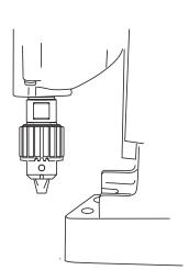
Thread the 3-Jaw Chuck onto the Spindle Adapter keeping the supplied washers centered, until tight. Now thread the complete assembly up onto the bottom of the motor.
