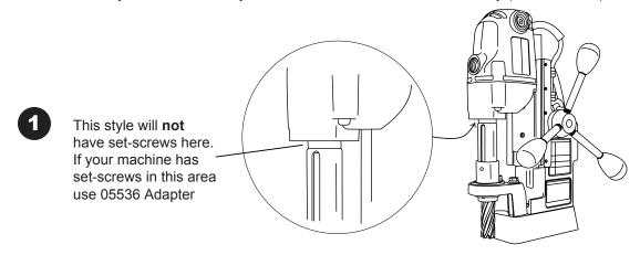
There are 2 methods to remove the Arbor Body Assembly from a threaded style spindle.
