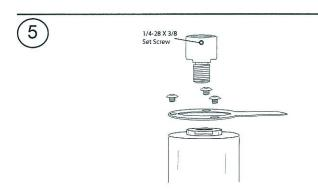
Install the Stop Arm to the Tap-Matic Assembly with the 3 Button Head Screws supplied with the Tap-Matic. Thread the Hex Adapter (05397) into the top of the Tap-Matic Assembly and install the 1/4-28 X 3/8 Set Screw (05628) into the side of the Hex Adapter.
