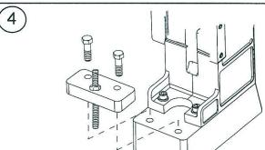
Install the 1/4-20 X 2-1/2 Set Screw (02432) and 1/4-20 Lock Nut (10859) into the Stop Block as shown. Mount the Stop Block Assembly to the Magnet with the supplied 3/8-24 Hex Bolts and tighten with a 9/16 Wrench.
