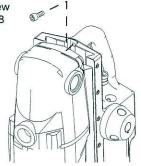
Verify that part number 40432 Stop Screw is installed. This Stop Screw should be threaded into the top of housing in front of the Motor Assembly as shown.
