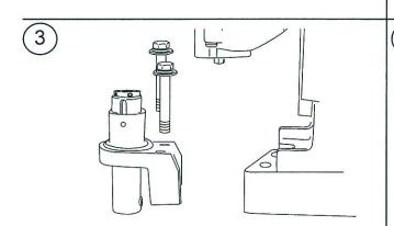
Remove both 3/8-24 Hex Bolts from the Front Support Bracket using a 9/16 Wrench.
