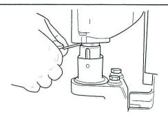
Remove the 1/4-28 X 3/8 set screws from the top of the Arbor Body with a 1/8" Hex Wrench.
