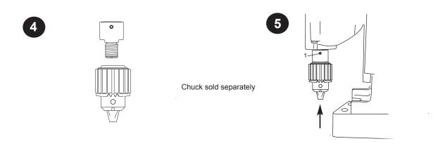
Thread the 3-Jaw Chuck onto the Spindle Adapter until tight. Now slide the complete assembly up onto the Hex Spindle at the bottom of the motor. While pushing up on the Spindle Adapter / Chuck Assembly, turn the set screw in at the top of the Adapter until tight; as shown in Fig.5.
