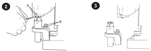
Remove the set screws (A) from the top of the Arbor Body and the Front Support Bracket Bolts (B) from the front of the Magnet. Once these are removed the Arbor Body Assembly can be removed from the Drill Assembly.
