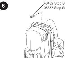
,40432 Stop Screw SHC 1/4-28 X 3/8 to use with the HMD904 or HMD908. 05357 Stop Screw SHC 1/4-28 X 7/8 to use with the HMD925.
