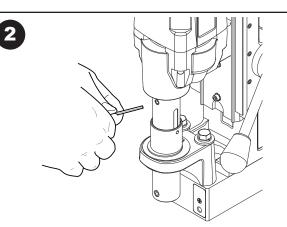
Remove the 5/16-18 x 3/8 set screw from the top of the Arbor Body with a 1/8" Hex Wrench.
