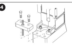
Install the 1/4-20 x 2-1/2 Set Screw and 1/4-20 Lock Nut into the Stop Block as shown. Mount the Stop Block Assembly to the Magnet with the supplied 3/8-24 Hex Bolts and tighten with a 9/16 Wrench.
