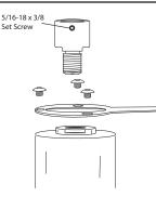
Install the Stop Arm to the Tap-Matic Assembly with the 3 Button Head Screws supplied with the Tap-Matic. Thread the Slot Drive Adapter into the top of the Tap-Matic Assembly and install the 5/16-18 x 3/8 Set Screw into the side of the Slot Drive Adapter.
