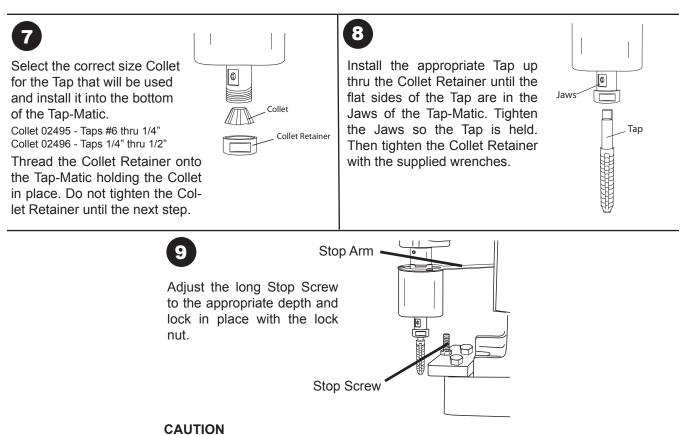
When the Tap is working down into the material the Stop Arm will rotate and make contact with the Drill Housing on the opposite side that is shown. When the Tap direction changes and the Tap is working out of the material it will rotate again to the opposite side. Keeps hands clear of the Stop Arm while operating.
