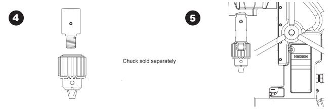
Thread the 3-Jaw Chuck onto the Spindle Adapter until tight. Now slide the complete assembly up onto the Slot Spindle at the bottom of the motor. While pushing up on the Spindle Adapter / Chuck Assembly, turn the set screw in at the top of the Adapter until tight; as shown in Fig. 5.
