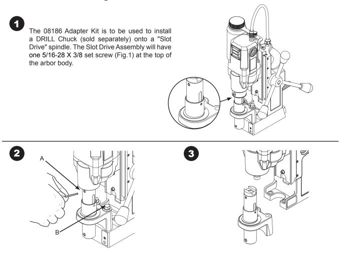
Loosen the set screw (A) from the top of the Arbor Body and the Front Support Bracket Bolts (B) from the front of the Magnet. Once these are removed the Arbor Body Assembly can be removed from the Drill Assembly.
