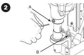
Rotate the Arbor Body so the 5/16-18 x 3/8 set screw inside, aligns with the hole in the Coolant inducer. Insert the 5/32" Hex Wrench and turn the inside set screw 1 full turn counterclock-wise or until loose.
