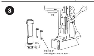
Remove both 3/8-24 x 3" Hex Bolts from the Front Support Bracket using a 9/16" wrench. Now the entire Arbor Body Assembly can be removed.
